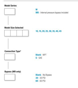
This is a partial flow pressure bypass only. It is not designed to be a full flow system bypass.
